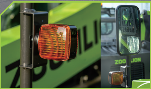
Optional turn signals and exterior rearview mirrors They do not move with the lifting arm, making it easy to observe the situation at the back of the machine at any time and keeping you safe.
